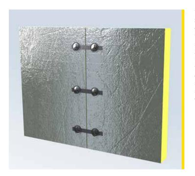
The different **U SeaProtect® Slab 66** panels are interconnected by steel connecting bridges (maximum spacing approximately 200 mm). Connecting bridges are used for both vertical and horizontal joints and consist of steel pins, washers and perforated steel strips on both sides of the extension.
