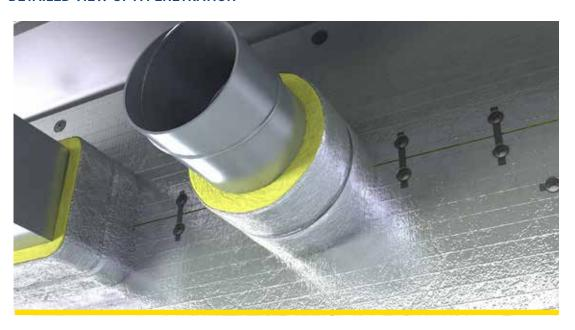
The passage of pipes, electrical cables and ventilation ducts is authorised if they are protected with **U SeaProtect® Roll 46 Alu1** with a thickness of 30 mm to maintain the fire integrity of the B-15 wall extension.
