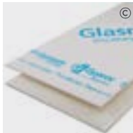
Glasroc® X Sheathing Board 12.5mm A high performance gypsum sheathing board with mould resistant properties. Use it to provide external weather protection prior to the installation of the finished exterior façade system.
